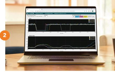
Every rig has a "flowback fingerprint", which refers to the expected Volume and Flow readings when the pumps are turned off and fluid returns to the tanks. Monitoring flowback is one of the only ways to catch potential gain/loss issues during pumps-off events.
