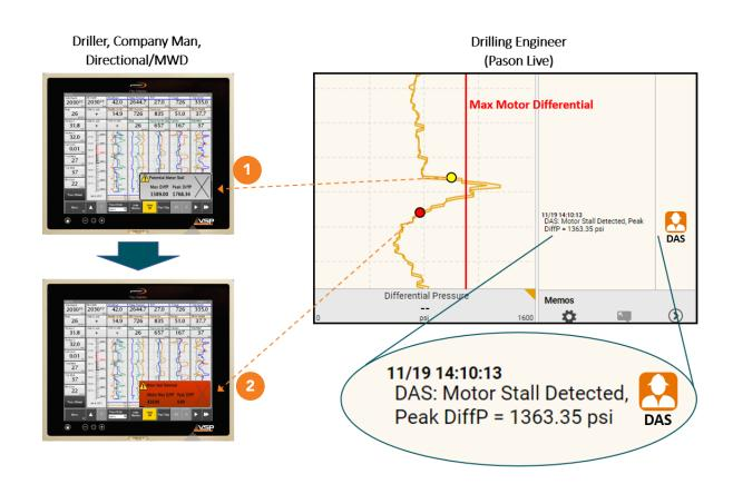
ExxonMobil DAS is technology licensed from ExxonMobil Upstream Research Company and deployed on Pason's AutoDriller technology platform for rigs with brakehandle or AC controlled drawworks.
